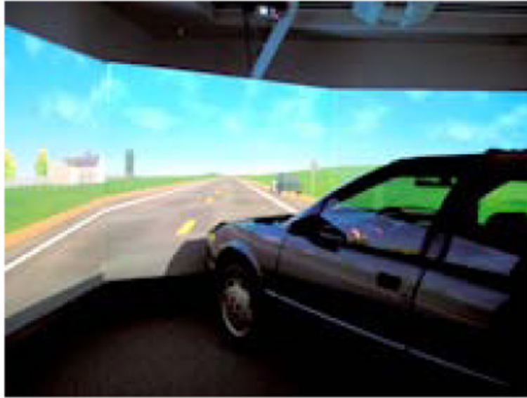
FIGURE 2. View of the Simulator for Interdisciplinary Research in Ergonomics and Neuroscience (SIREN Cab and Front Screens
